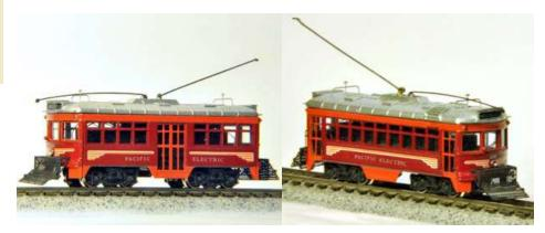
**Photo 2:** Showcase Miniatures version of a 600-series Pacific Electric "Hollywood" car on a Kato B-B power chassis; note the pole in the image on the right; it uses the old reliable NCAT design of shoe (or "trolley") to track overhead wire.
